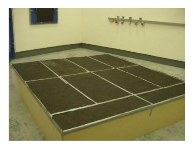
Figure 4.3: Test sample fitted to the Type E mounting.
